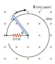
electrical contact with the wire at all times. The wire and the bar have negligible resistance. A uniform magnetic field exists everywhere, is perpendicular to the plane of the circle, and has a magnitude of B. Which of the following shows the magnitude of the current as a function of  $\theta$ ?
